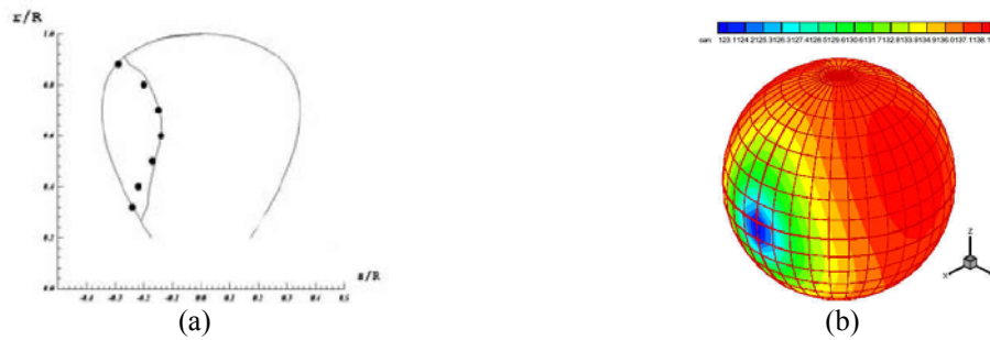
Figure 5: Cavity Planform and Blade Surface Cavitation Noise Directivity 3D Contour. (a) Cavity Planform for Model Propeller (b) Blade Surface Cavitation Noise Directivity
