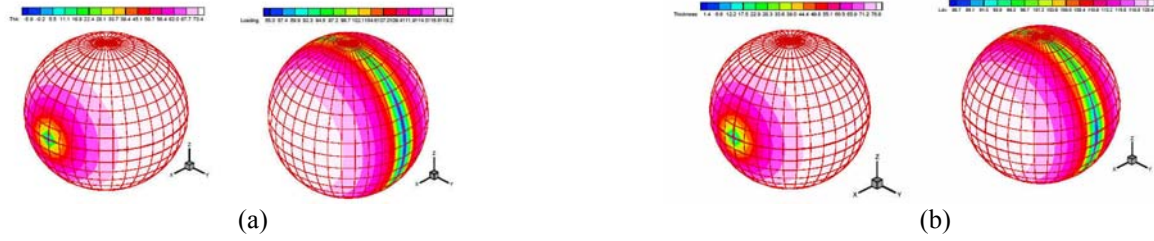
Figure 2 : Non-Cavitation Noise Directivity 3D Contour. (a) Single Propeller, Thickness Noise and Loading Noise. (b) Ducted Propeller, Thickness Noise and Loading Noise.
